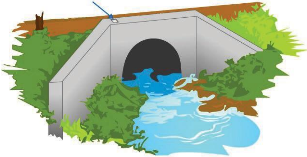
Figure 5-15 - Points on existing structures used as bench marks.
